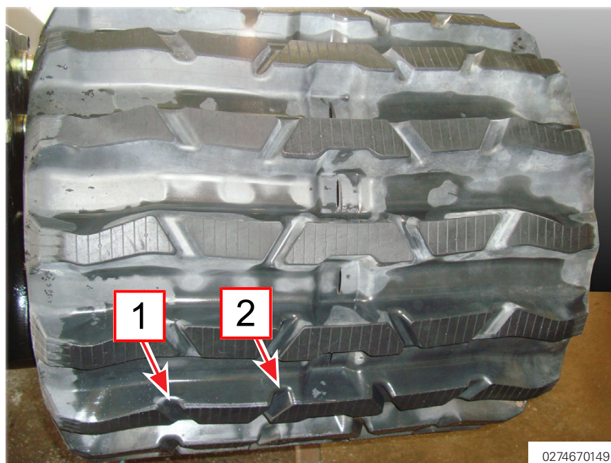
Illustration 26: Rubber Track Wear
