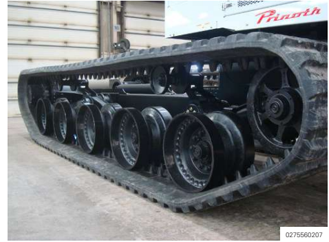
Illustration 213: Track under tension (generic image)
