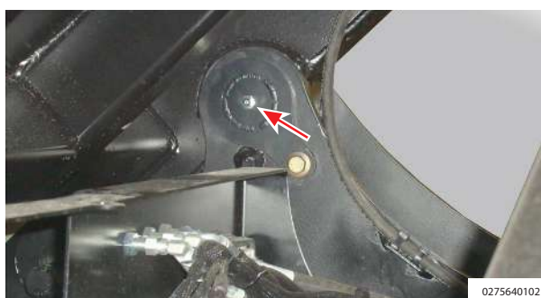
Illustration 239: Lubrication points of the dump body hinges (one left, one right)
