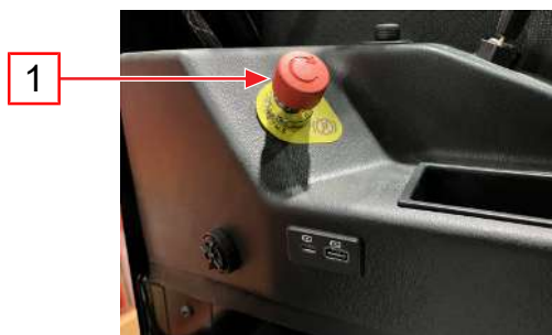
Illustration 42: Emergency stop switch
