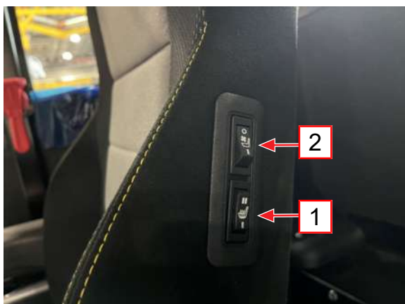
Illustration 104: Heating and cooling
