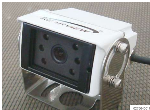
Illustration 130: Exterior camera with low light capability
