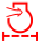
Illustration 195: Icon indicating restriction on the engine air filter
