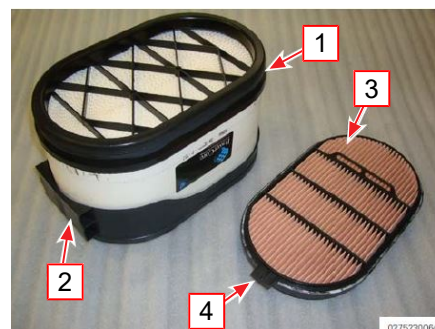
Illustration 191: Replacing the Engine Air Filter
