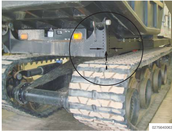
Illustration 228: Backlash measurement location
