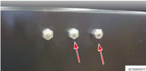
Illustration 240: Lubrications points of the vehicle slewing bearing Pinion (swing system)
