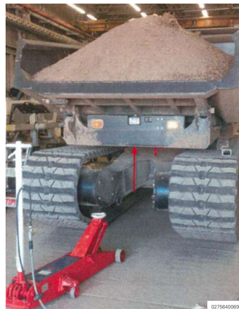
Illustration 226: Floor jack and rear of upper frame
