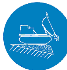
Illustration 178: Do not carry out dumping operation on a slope
