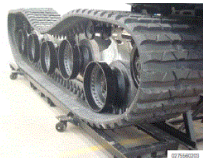
Illustration 212: Track installed but not yet under tension (generic image)
