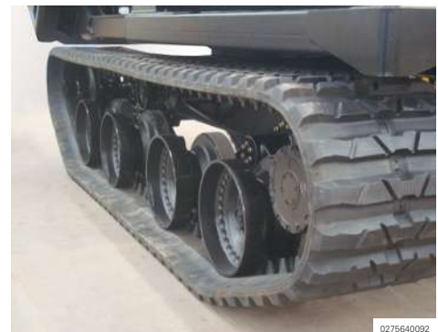
Illustration 209: Correct track tension
