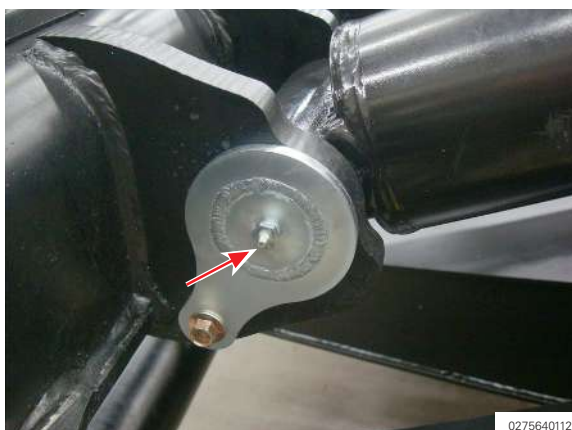
Illustration 238: Lubrication point of the dump body cylinder lower hand (one left, one right)
