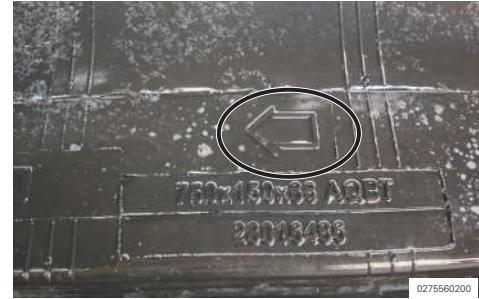
Illustration 210: Indication of rotation direction on internal surface of track
