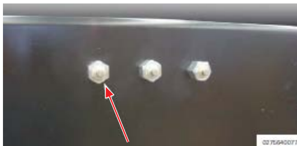
Illustration 237: Lubrication point of the dump body cylinder upper hands (one fitting for both cylinder hands)
